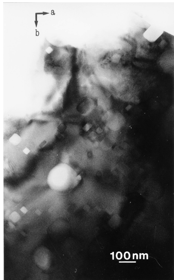
Fig. 6. Bright field image of the ab -plane of sillimanite annealed for 18 h.
